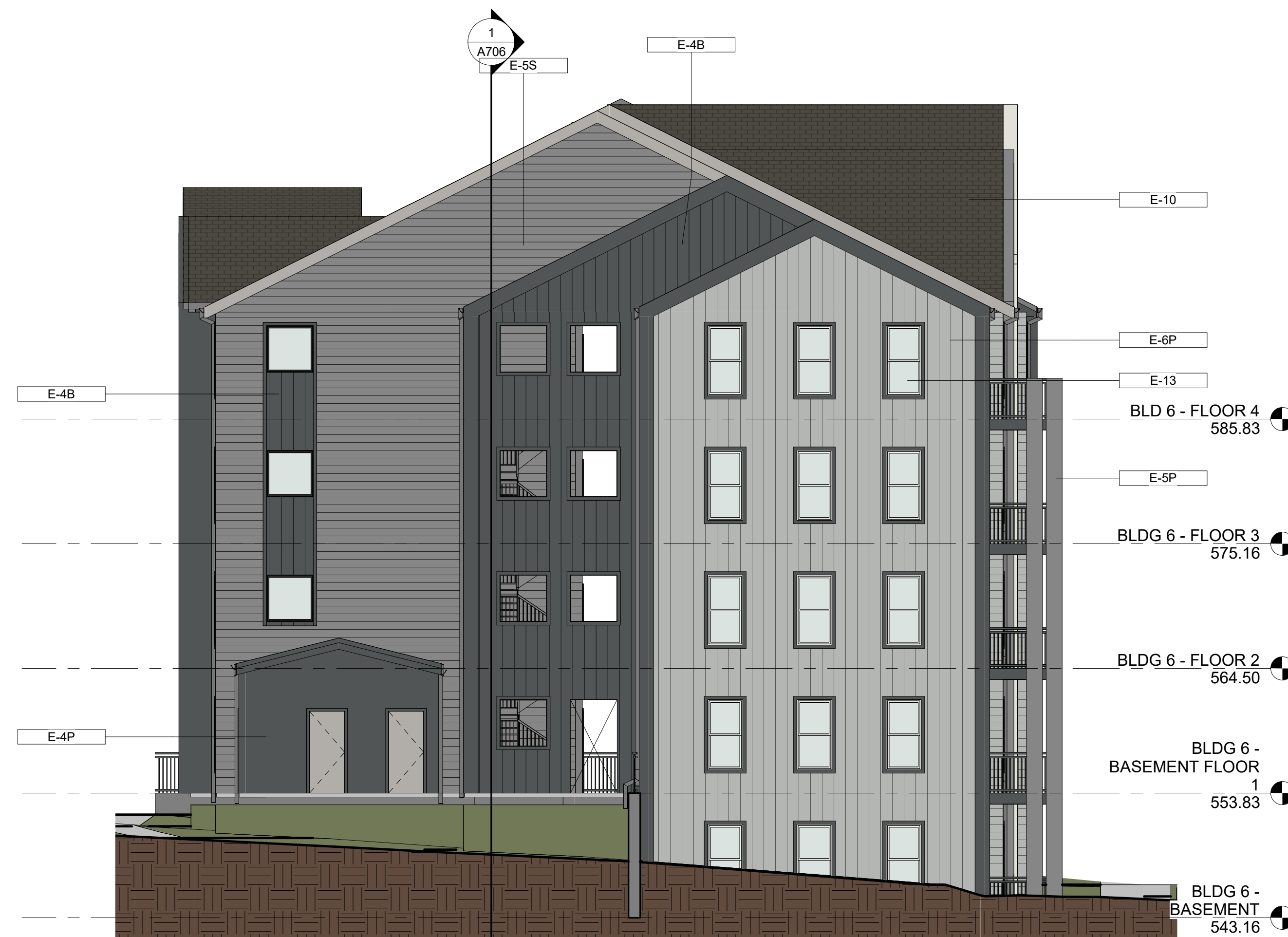
2 BUILDING 6 (TYPE 5) - NORTH ELEVATION 1/8" = 1'-0"
